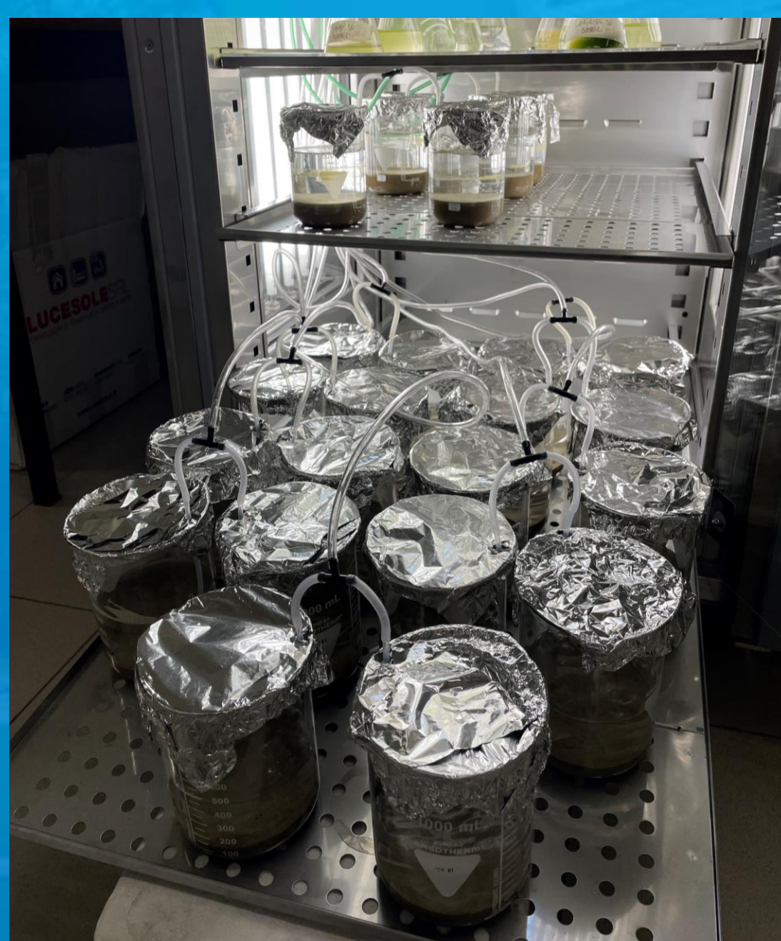
Fig. 2 Microcosms used for the experiment of exposure of bioplastic to marine sediment
