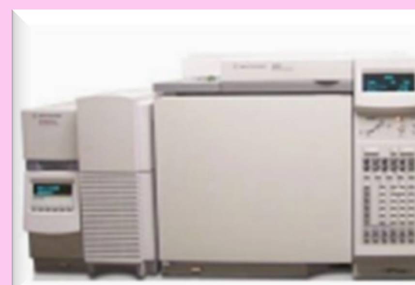
GC-MS: Agilent 6890 GC + 5973N quadrupole selective detector.
