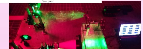
**OPTICAL VISUALIZATION OF A SALT GRADIENT SOLAR POND INTEGRATED WITH PCM**
