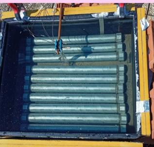
Abstract: In this work, a SGSP with PCM (RT35 HC) and a traditional one were designed, built and tested to evaluate the different performance. Then the effect of different melting temperatures (RT35 HC and RT44 HC) was experimentally investigated.
