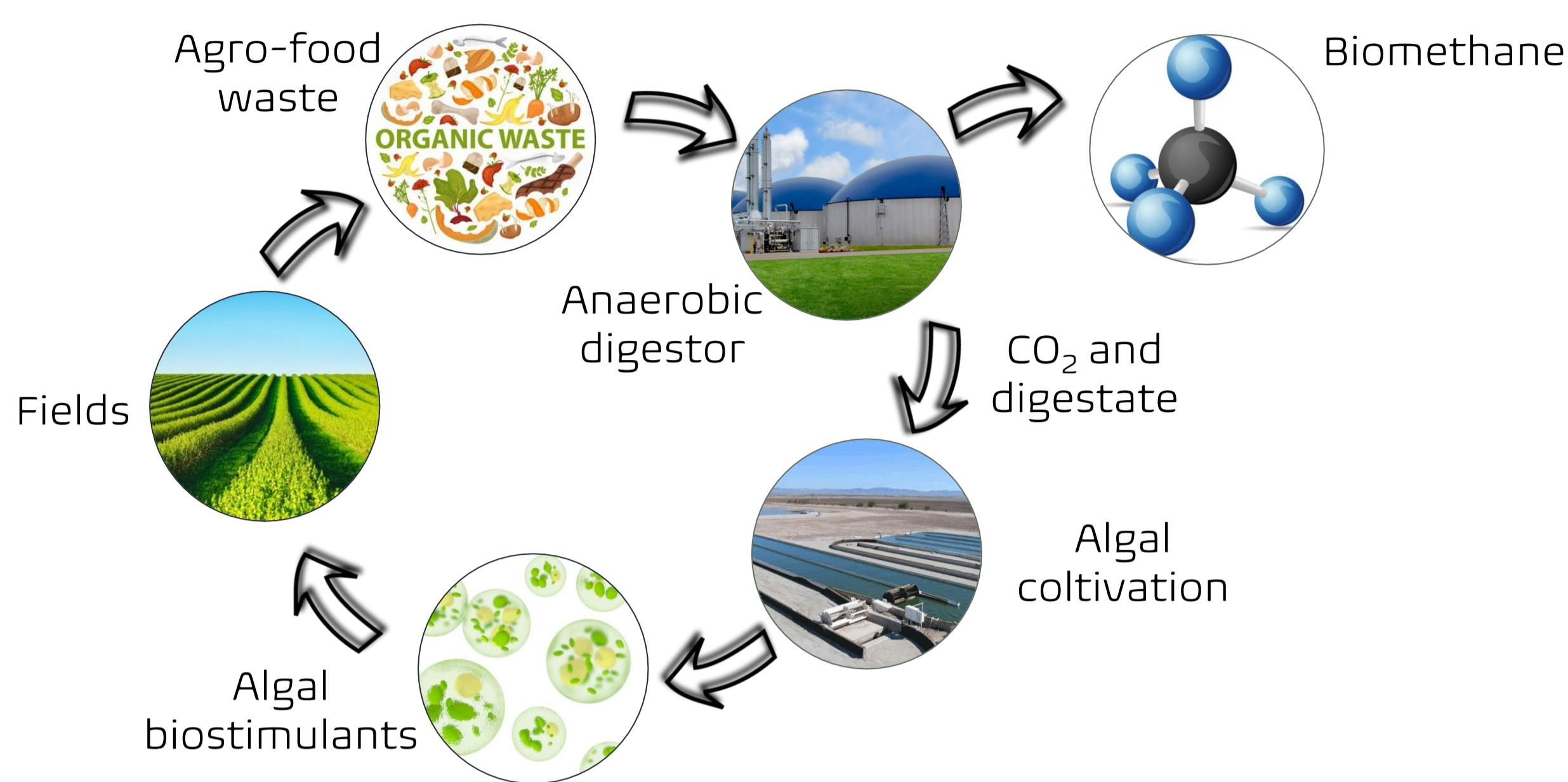
The main goal of the PhD project is to realise a «field-to-field» circular process where microalgae are used to remediate wastewaters (digestate) and CO<sub>2</sub> coming from the anaerobic digestion of organic waste and the upgrading of biogas to biomethane. The algal biomass produced during the remediation will be used to biostimulate crops grown on the same fields the waste came from.
