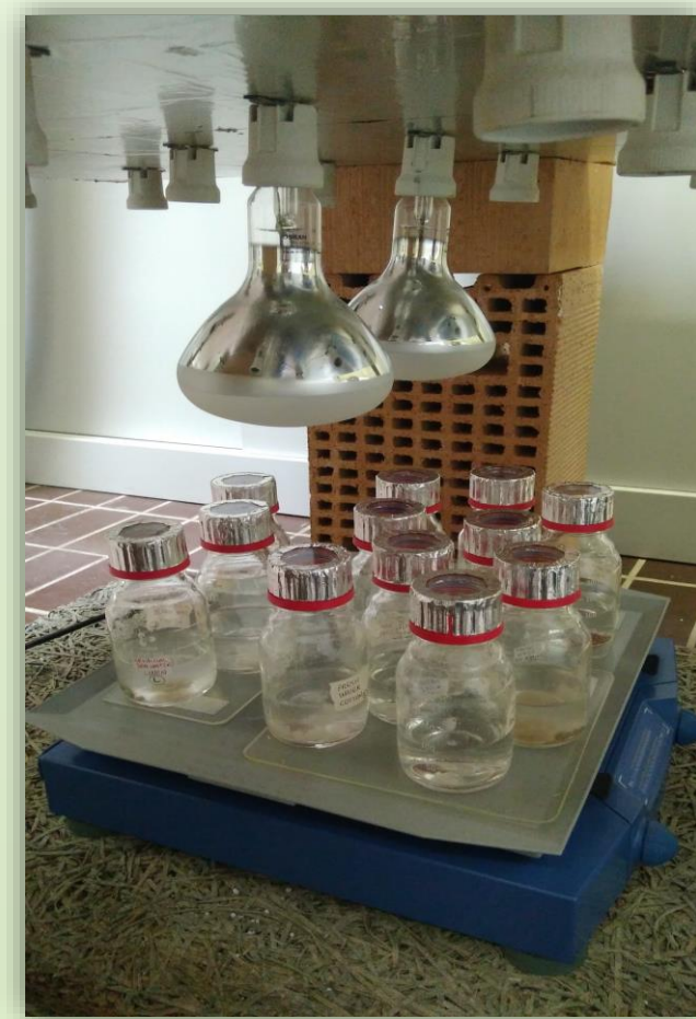
Fresh water and artificial sea water bottles filled with 1g/L of textile microfibers under the solar simulator lamp.
