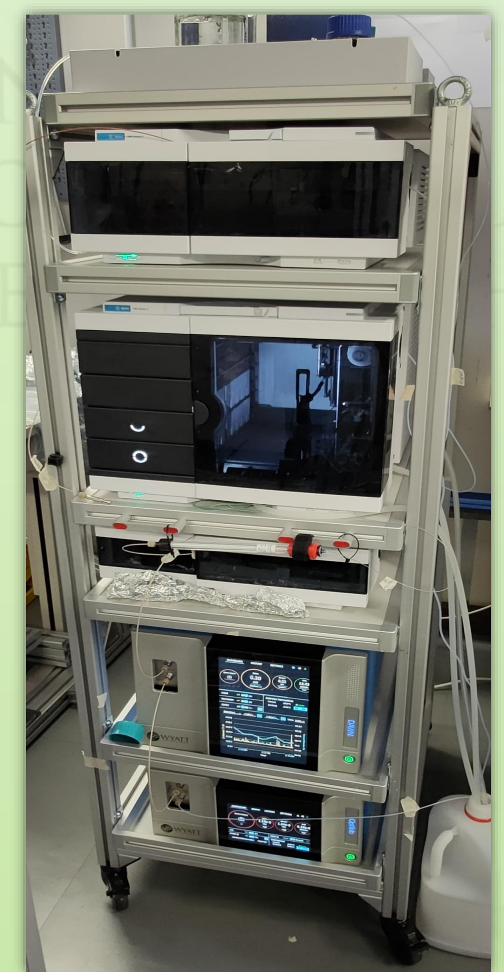
HPLC Agilent 1260II Infinity with Wyatt Mals detectors 18 angles, Quasi-Elastic Light Scattering – DLS and DRI Optilab Detector
