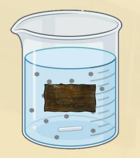
Treatment with Calcium Carbonate (CaCO<sub>3</sub>) NPs by immersion on non-acidificated wood
