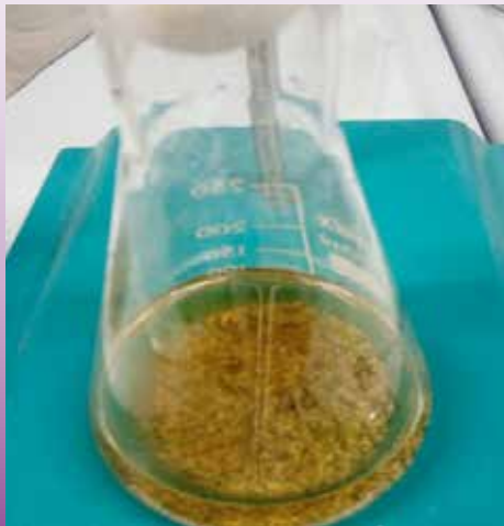
Bioleaching experiment with acidophilic bacteria
