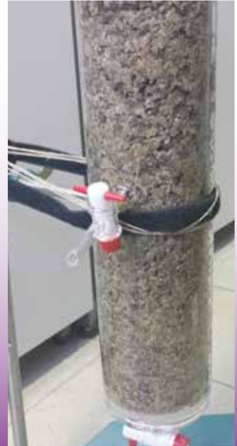
Glass fixed bed column packed with algae
