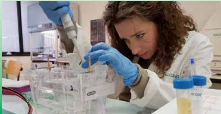
Load samples in to SDS-PAGE
